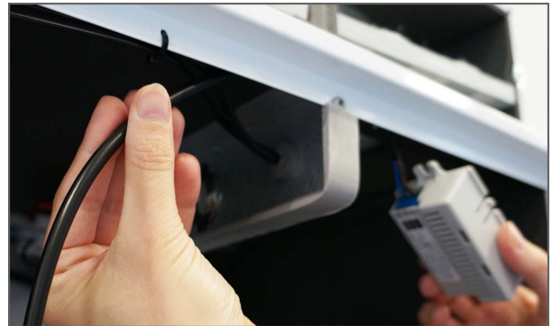
4. Run the wire from the CO 2 sensor through this recess.
