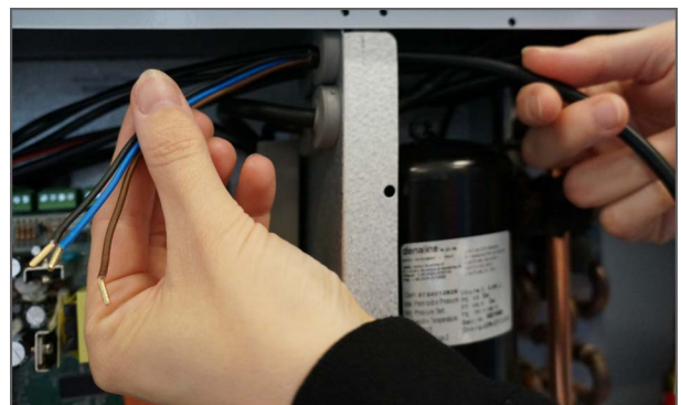
6. Run the wire from the CO 2 sensor through the cable grommet to the automation. Wire is subsequently tied up with cable strips.
